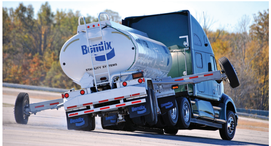
» A truck, shown on a demonstration track, with its electronic stability control system turned off (above) and on (below).
