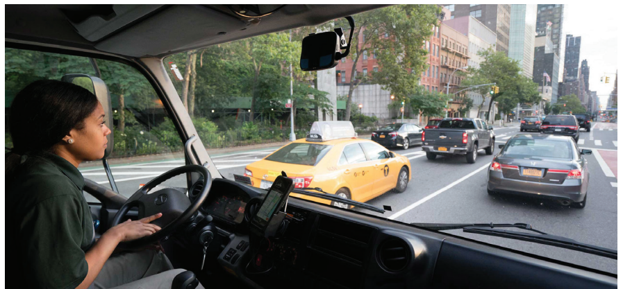
» Forward monitoring and driver monitoring cameras (above and below) mounted inside the cab.
