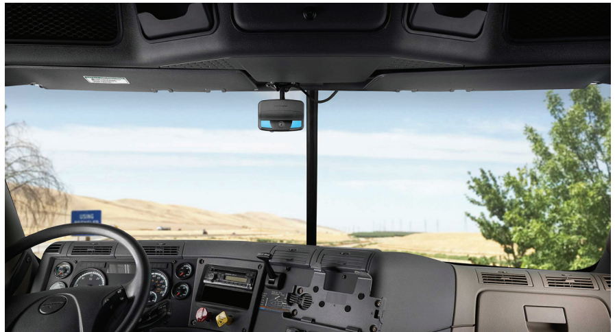
» Forward monitoring and driver monitoring cameras (above and below) mounted inside the cab.
